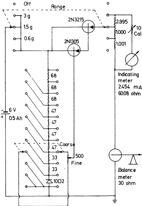
Fig. 1. Schematic diagram of the electromagnetic balance. All resistor values in ohms.
