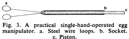
Fig. 3. A practical single-hand-operated egg manipulator. a. Steel wire loops. b. Socket. c. Piston.
