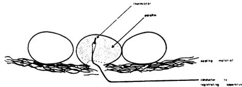
Fig. 1. Cross-section of the nest, showing the thermistor mounted inside one egg.
